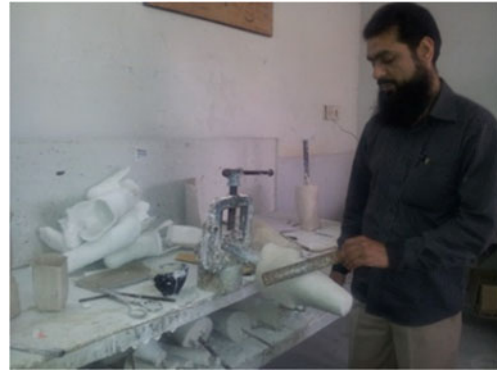
Fig. 4 Rectification of mould for manufacturing of the socket of the prosthesis
