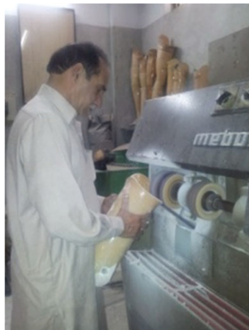
Fig. 5 Final shaping of the socket of an above knee prosthesis
